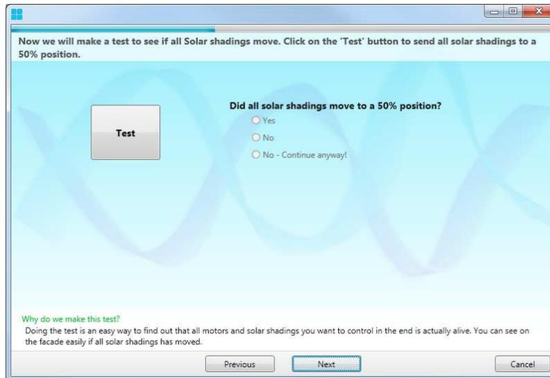
Picture 14: Make New Configuration – Test motors found.
