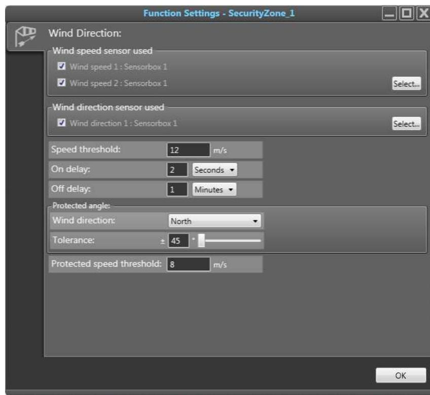
Picture 81: Function Settings – the Wind Direction function.
