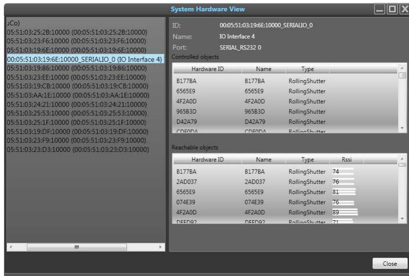
Picture 67: System Hardware View - Showing the SubCos and the motors.
