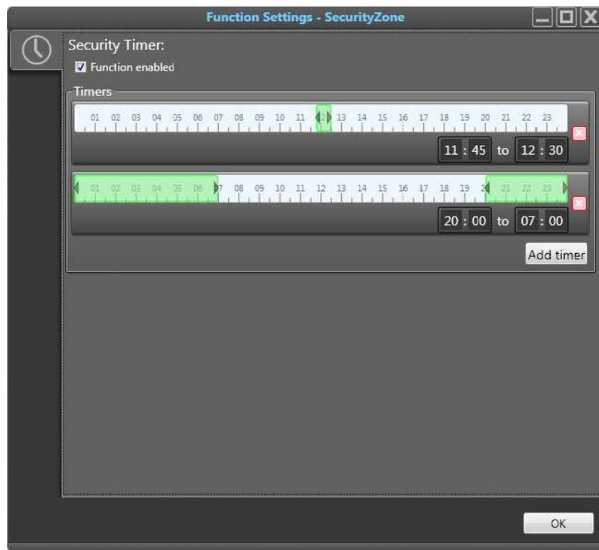
Picture 85: Function Settings - Security Timer - Solar shadings blocked during lunch and night.
